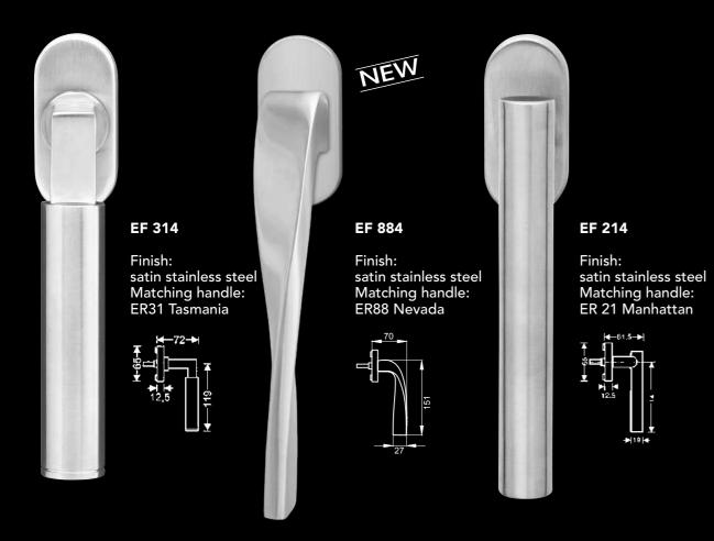
Rotates in 4 positions at 90° Hole distance: 43 mm, Fixing: M5 with fixing lugs Ø 10 mm  $\Box$  7 mm spindle, standard length 35 mm, also available in 30 and 40 mm for wooden/plastic windows Cap: 65 x 30 x 12 mm
