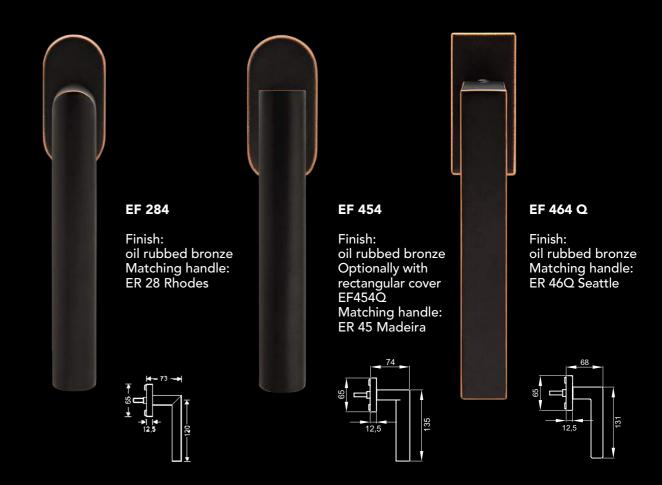
Also available in cosmos black\*. Rotates in 4 positions at 90° Hole distance: 43 mm, Fixing: M5 with fixing lugs Ø 10 mm  $\Box$  7 mm spindle, standard length 35 mm, also available in 30 and 40 mm for wooden/plastic windows Cap: 65 x 30 x 12 mm
