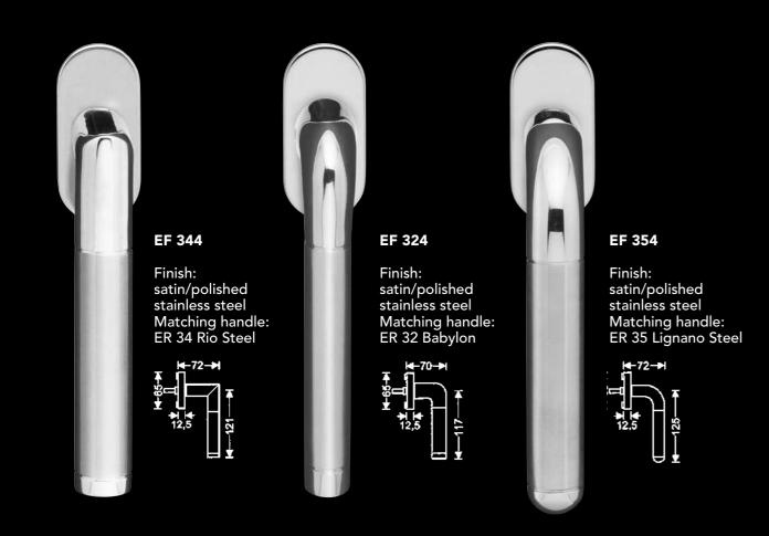
Rotates in 4 positions at 90° Hole distance: 43 mm, Fixing: M5 with fixing lugs Ø 10 mm  $\Box$  7 mm spindle, standard length 35 mm, also available in 30 and 40 mm for wooden/plastic windows Cap: 65 x 30 x 12 mm
