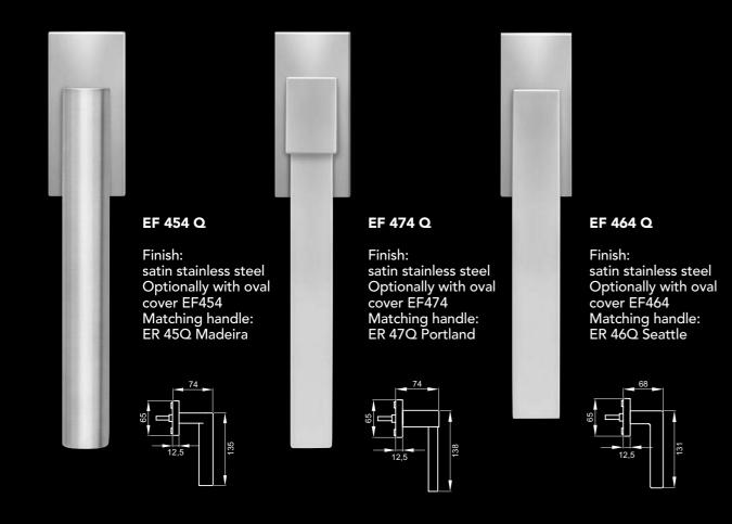
Rotates in 4 positions at 90° Hole distance: 43 mm, Fixing: M5 with fixing lugs  $\emptyset$  10 mm  $\square$  7 mm spindle, standard length 35 mm, also available in 30 and 40 mm for wooden/plastic windows Cap: 65 x 30 x 12 mm
