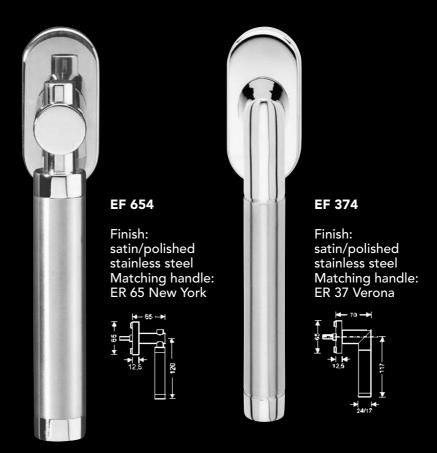
Rotates in 4 positions at 90° Hole distance: 43 mm, Fixing: M5 with fixing lugs Ø 10 mm  $\Box$  7 mm spindle, standard length 35 mm, also available in 30 and 40 mm for wooden/plastic windows Cap: 65 x 30 x 12 mm
